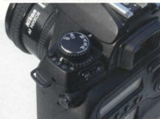
Several new controls have been added around the eye-level viewfinder. Previously, there was a diopter control for eyeglass wearers and an AE lock button. The S2 Pro has the same diopter control and AE lock, but has added the AF lock and controls for Matrix, spot, and center weight metering.
